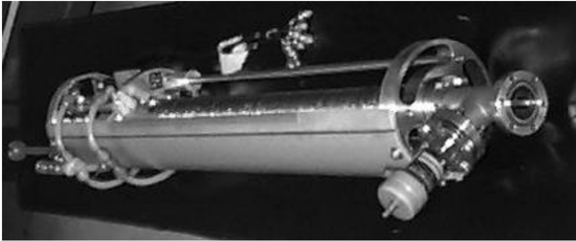
Figure 2. A photograph of an FRC Langmuir probe head which is attached to a reciprocating drive. The probe head is at the far right hand side.
